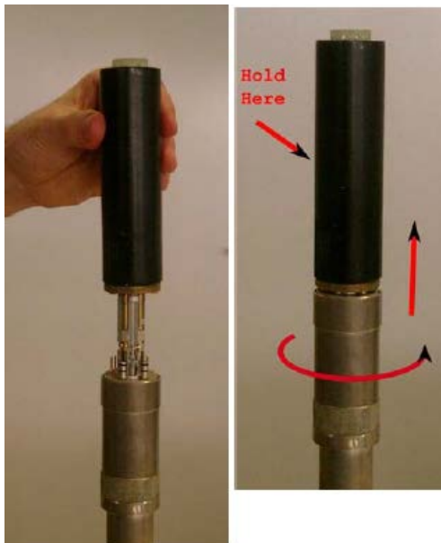
Figure 11.3: Mounting the Gradient System
