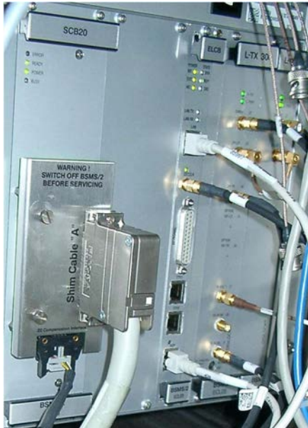
Figure 12.10: BSMS-2 to B0-2 Adaptor Board, Mounted on the Most Right SCB20 Module
