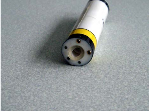
Figure 11.4: Bottom View Showing Silicon Rubber Sealing
