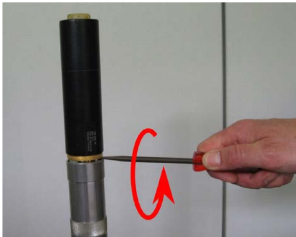
Figure 11.1: Gradient Coil Removal
