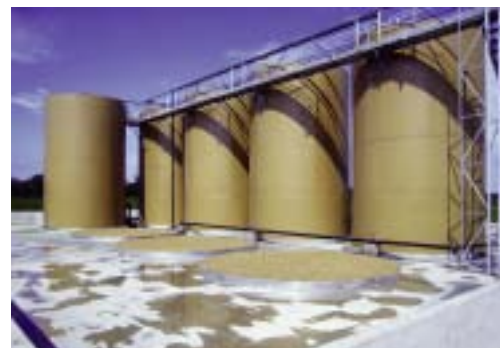
Picture 4: Production containers-750 bbl tanks
