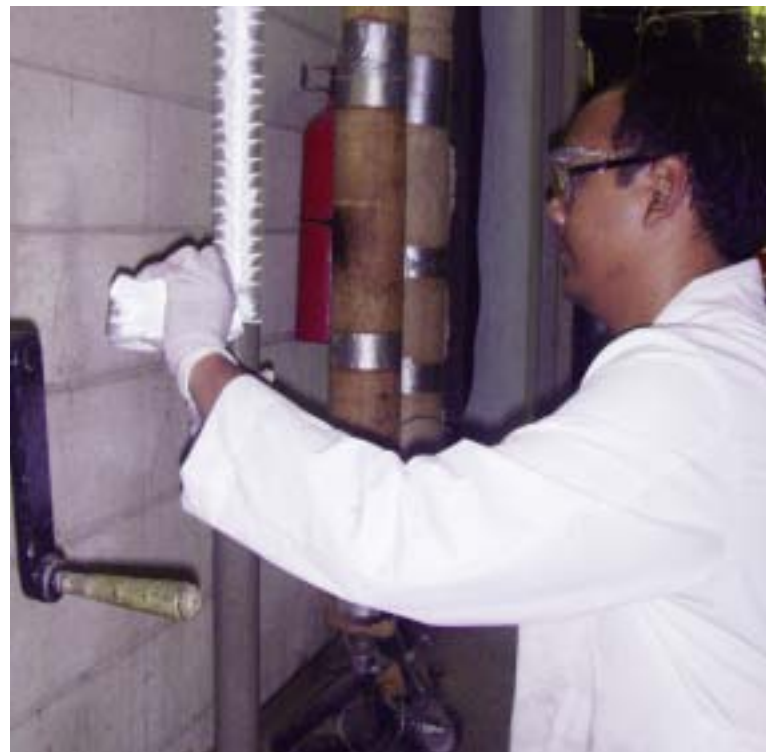
Ruiz wrapping a 6' core with glass fiber tape
