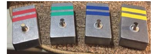
Device pedal hardware (Controls Actuation of Chords)
